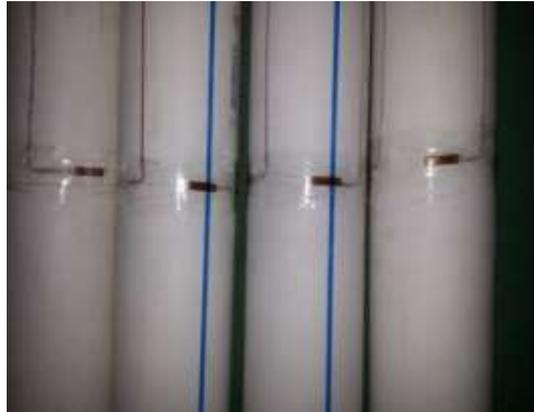
*Figure 2: The pipes with strain gauges used in experiments.*
