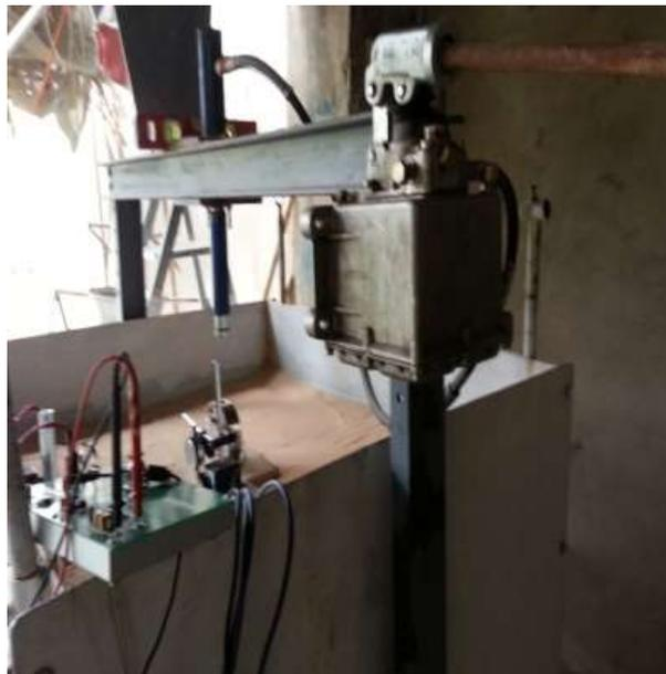
*Figure 3: The soil box and frame used in static test.*
